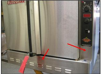
3. Disconnect the gas supply line to gas manifold and remove the two bolts that hold the gas manifold in
