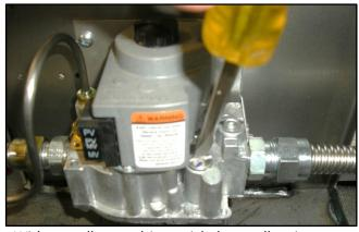
With a small screwdriver, pick the small spring out of the hole in the valve under the gas adjustment
